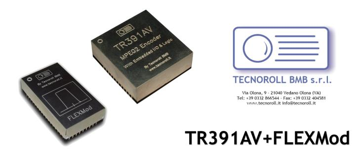
4 channell MPEG-2 encoder + multiplexer + DVB modulator
